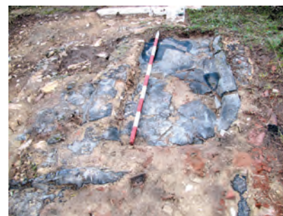
Fig. 31. C9: floor and wall foundations covered in bitumen.
